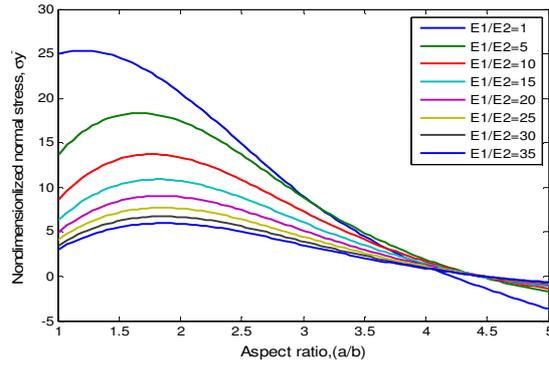
**Figure 4: Nondimensionalized Normal Stress ( $\sigma_y$ ) Versus Aspect Ratio ( $a/b$ ) for Different Modulus Ratios  $E_1/E_2$**
