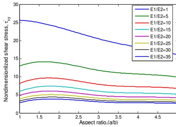
**Figure 5: Nondimensionalized Shear Stress ( $\tau_{xy}$ ) Versus Aspect Ratio ( $a/b$ ) for Different Modulus Ratios  $E_1/E_2$**
