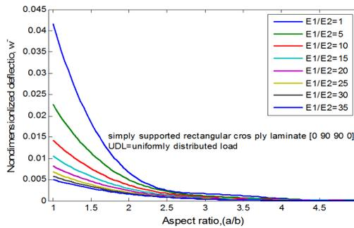
Figure 2: Nondimensionalized Maximum Transverse Deflection (W) Versus Aspect Ratio (a/b) For Different Modulus Ratios E1/E2
