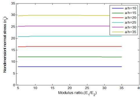
Figure 7: Nondimensionalized Normal Stress ( $\sigma_y$ ) Versus Modulus Ratio ( $E_1/E_2$ ) For Different Side to Thickness Ratios  $a/h$
