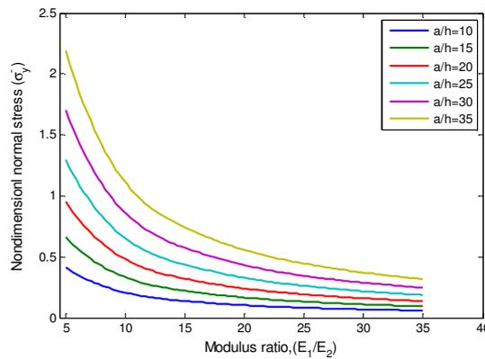
Figure 8: Nondimensionalized Normal Stress ( $\sigma_x$ ) Versus Modulus Ratio ( $E_1/E_2$ ) For Different Side to Thickness Ratios  $a/h$
