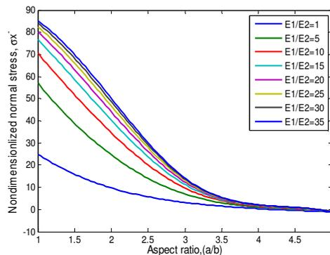
Figure 3: Nondimensionalized Normal Stress ( $\sigma_x^-$ ) Versus Aspect Ratio (a/b) for Different Modulus Ratios E1/E2
