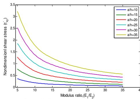
Figure 9: Nondimensional Shear Stress ( $\tau_{xy}$ ) Versus Modulus Ratio ( $E_1/E_2$ ) For Different Side to Thickness Ratios  $a/h$
