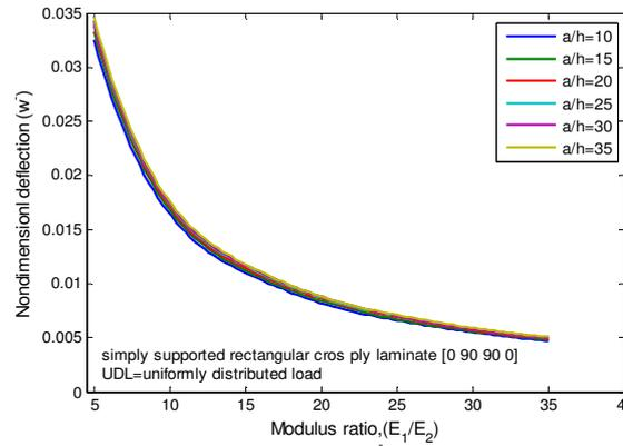
**Figure 6: Nondimensionalized Deflection ( $w$ ) Versus Modulus Ratio ( $E_1/E_2$ ) for Different Side to Thickness Ratios  $a/h$**
